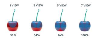
The Total View system analyzes more of the cherry's surface. It also removes false positives which can be caused by the cherry's stem being classified as a defect.
